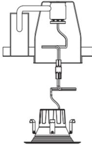
4. Carefully route wires into fixture, simply slide the trim and metal friction clips into the housing. *(Fig.4)*
