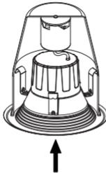
5. Push the LED trim into the housing until flush with ceiling. *(Fig.5)*
